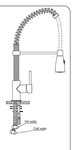
Make sure the installation holes are in the correct size. Install the lavatory and pop-up waste as shown in the drawing. Connect the main body and water supply pipe with water inlet pipe
